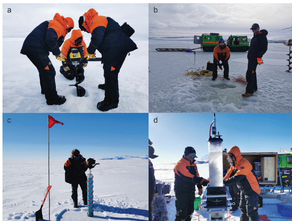
Fig. 3. Sampling for eDNA and live mixed samples in Antarctica, including (A) sea ice auger to collect brine samples, (B) plankton net deployed below ice, (C) SIPRE core drill for sea ice core samples and (D) sub-ice platelet layer (SIPL) sampler. Image credits: Jacqui Stuart.
